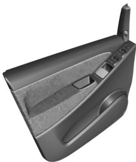
Figure 10 Piece of a car door molded with resin reinforced with sisal fibers.
